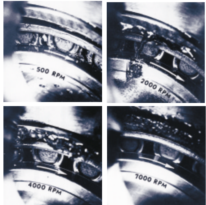
Pumping effect of a tapered roller bearing
